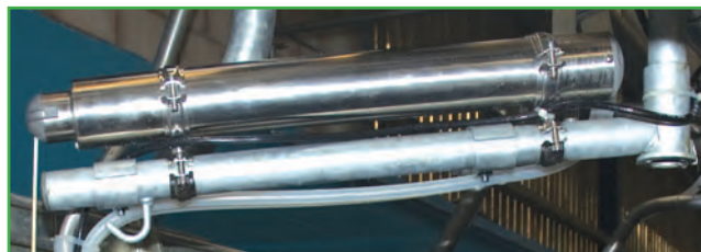
5019MK ACR Cylinder with 5015 Angled Swing Arm in parlour
