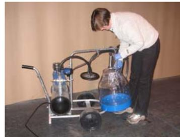
Repeat steps 1—7 using hot water (3 gals, 50°C) with circulation detergent. Then finally repeat again with a cold water rinse. **Keep motor running.**
