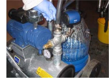
Turn off the vacuum supply to the bucket. Above shows the vacuum ON position.
