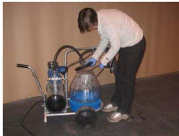
Remove the lid and take the bucket off the milker. Dispose of the cold rinse water. Replace the bucket and close the cluster shut off, turn the bucket vacuum back ON.
