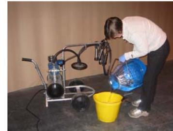
After the warm water with detergent has passed through save it back in a bucket before placing the bucket back on the milker.
