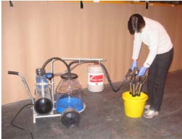
Immediately after the completion of milking the unit should be cleaned. Fill a bucket with approx 2 gallons of cold water.
