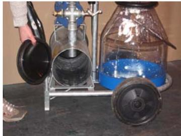
Remove the vacuum tank end covers, they are a push fit.
