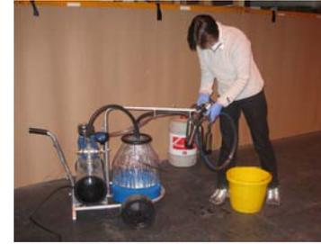
Hang the cluster back up leaving the shut off in the open position drawing air through the cluster and tubing.
