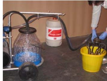
Open the cluster shut off valve slowly. Close and open the valve while the water is being drawn up to create a slugging effect and turbulence, to wash all surfaces.
