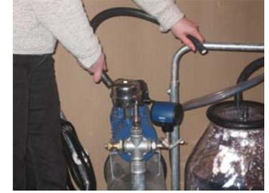
Remove the vacuum supply tube from the bucket lid and the stall tap.
