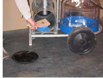
Clean the inside of the tank and the tank end covers and seals with detergent water.
