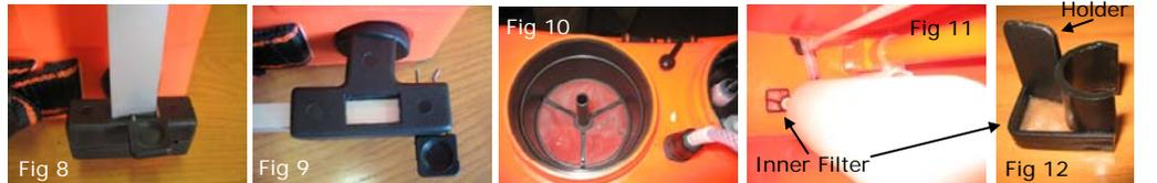
7. Prior to filling the Neptune the inner filter should be removed and cleaned. Unscrew the top cap that is NOT marked 'For Service Only', the filling filter should be removed and rinsed in clean water. This allows access to the tank, at the base of the pressure bottle is the inner filter which can be removed by pulling on the holder, this should then be removed and rinsed in clean water; reinsert the filters. Figs 10 to 12
