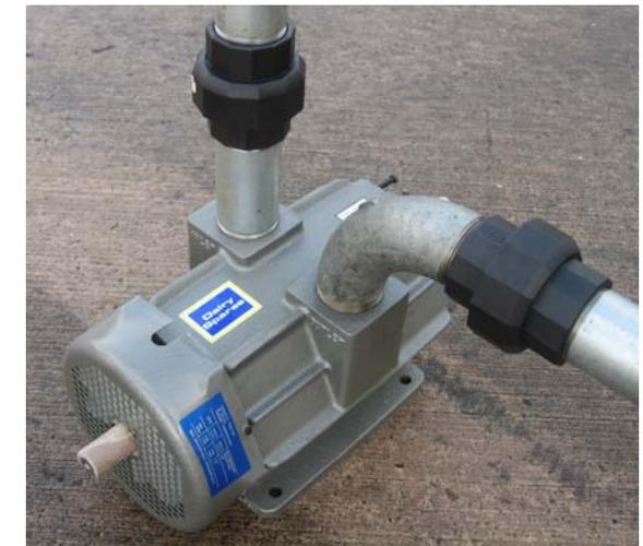
Using two unions on this vacuum pump; one the vacuum supply and the other to the exhaust.
