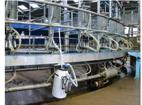
The DB28 bracket positions the bucket to allow it to pass underneath the entry bridge.
