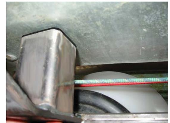
The DB29 bracket is spaced to permit unimpeded operation of the control cords.
