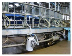
The DB28 bracket positions the bucket to allow it to pass underneath the entry bridge.
