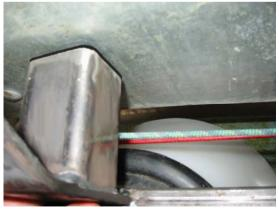
The DB29 bracket is spaced to permit unimpeded operation of the control cords.
