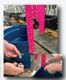
Using the marked holes, bolt the hook to the feeder and tighten with the 10 mm spanner and socket.
