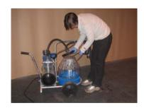
Remove the lid and take the bucket off the milker. Dispose of the cold rinse water. Replace the bucket and close the cluster shut off, turn the bucket vacuum back ON.
