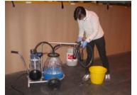
Hang the cluster back up leaving the shut off in the open position drawing air through the cluster and tubing.
