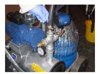
Turn off the vacuum supply to the bucket. Above shows the vacuum ON position.
