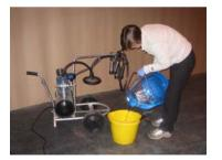
After the warm water with detergent has passed through save it back in a bucket before placing the bucket back on the milker.
