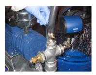
Open the vacuum supply to the bucket to allow the vacuum pump to draw air through the system and prevent reverse rotation on switch off.
