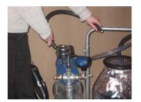
Remove the vacuum supply tube from the bucket lid and the stall tap.
