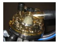
The motor running generates heat helping dry any moisture carried through on the air flow.
